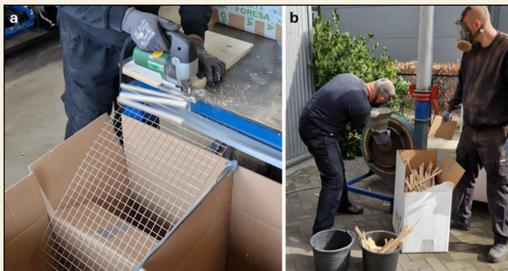
Figure a-b-c show the sizing and grinding of plywood and modified wood.
