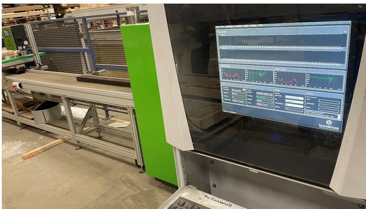
Figure 4. Crack detection device at Foreco
