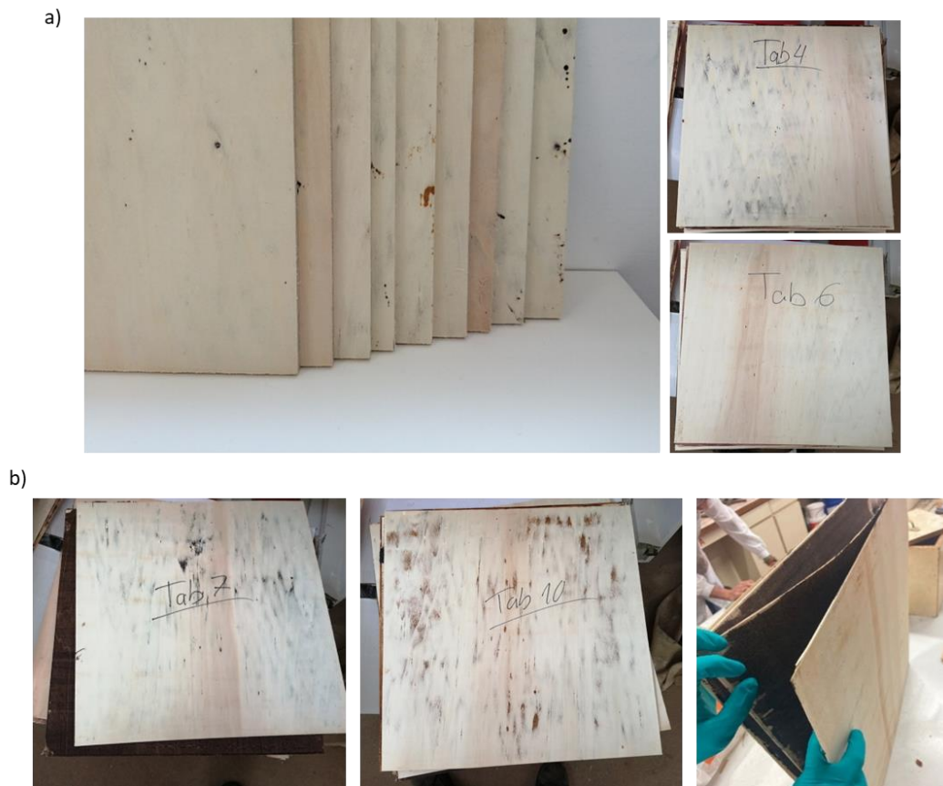
Figure 2. Plywood products a) obtained and b) unglued after pressing process.
