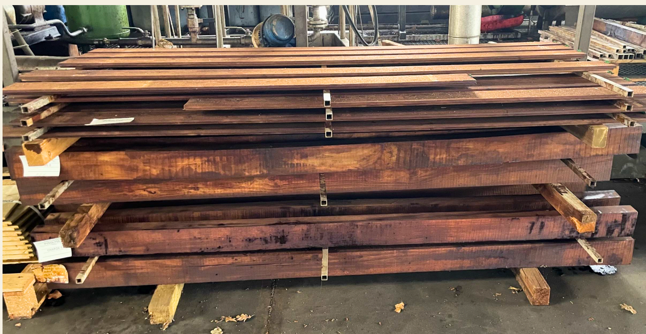
Figure 12: Wood samples at FORECO impregnated with an FPBO derived formulation
