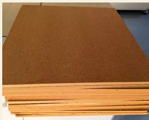
Figure 11: the sixteen 50x50cm MDF boards produced by FORESA Technologies
